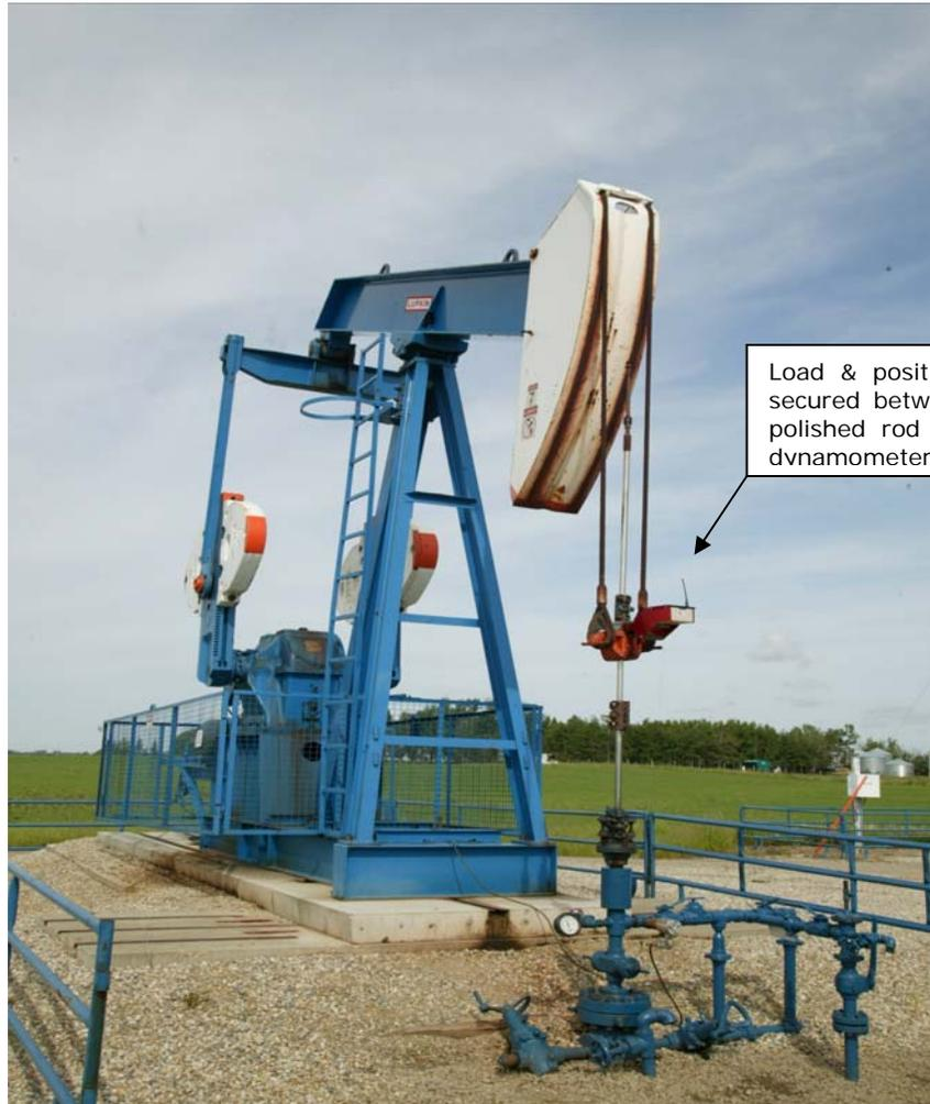
Load & position transducers are secured between carrier bar and polished rod safety clamp for a dynamometer test.
