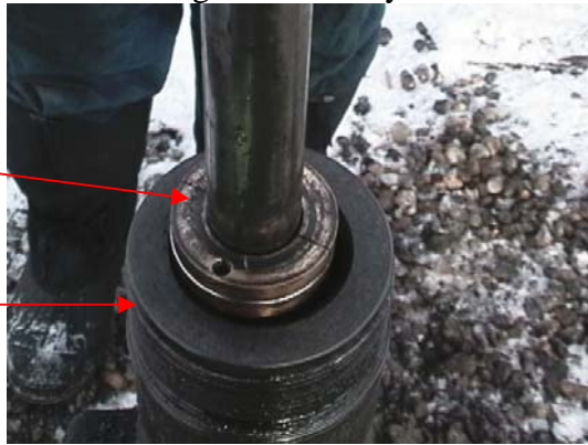
Above misalignment is easy to see before anything is taken apart and may be the problem.
