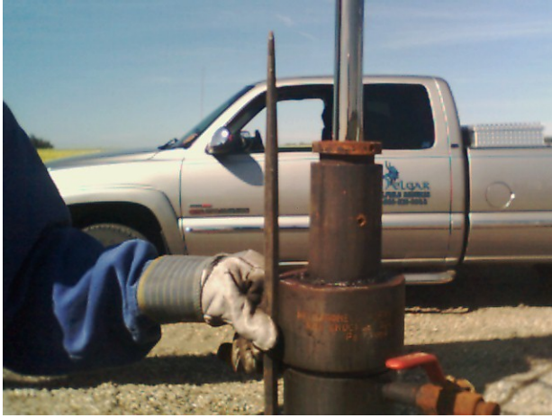
Above misalignment is easy to see before anything is taken apart and may be the problem.
